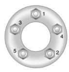
Tighten the wheel nuts firmly in a crisscross sequence as shown.
